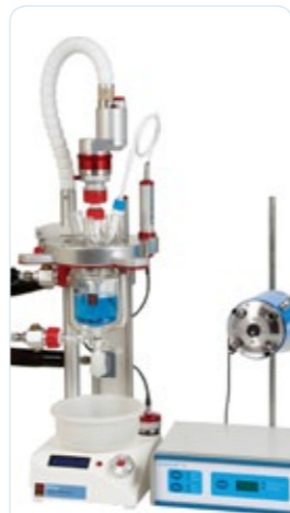
Atlas Sonolab Use ultrasound energy in crystallizations for narrow particle size distribution and polymorph control.
